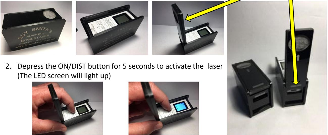
2. Depress the ON/DIST button for 5 seconds to activate the laser (The LED screen will light up)
